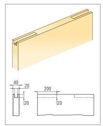
CLOISON: OSSATURE 2x48 mm
